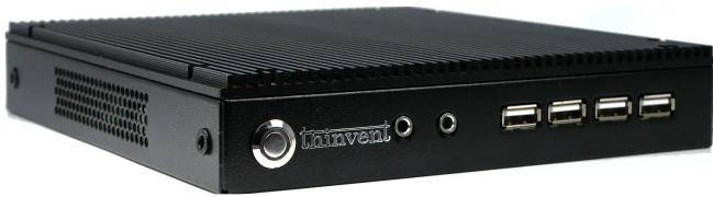
Thinvent® Industrial PC IPC1, Intel® processor N100 (4 core, up to 3.4 GHz, 6 MB cache), 32GB DDR4 RAM, 32GB SSD, 12V 2A Adapter, No WiFi, Thinux™ Embedded Linux, Thinvent® Keyboard and Mouse set
