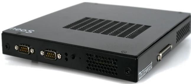
Thinvent® Neo S Thin Client, Intel® processor N100 (4 core, up to 3.4 GHz, 6 MB cache), 16GB DDR4 RAM, 32GB SSD + 32 GB MLC SSD, 12V 2A Adapter, No WiFi, Thinux™ Embedded Linux, Thinvent® Keyboard and Mouse set
