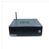
Thinvent® Neo R/4 Mini PC, Intel® processor N100 (4 core, up to 3.4 GHz, 6 MB cache), 64GB DDR4 RAM, 32GB SSD, 12V 2A Adapter, Dual Band WiFi, Thinux™ Embedded Linux
