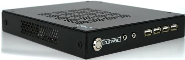
Thinvent® Treo Mini PC, Intel® processor N100 (4 core, up to 3.4 GHz, 6 MB cache), 4GB DDR4 RAM, 32GB SSD, 12V 5A Adapter, No WiFi, Thinux™ Embedded Linux, Thinvent® Keyboard and Mouse set
