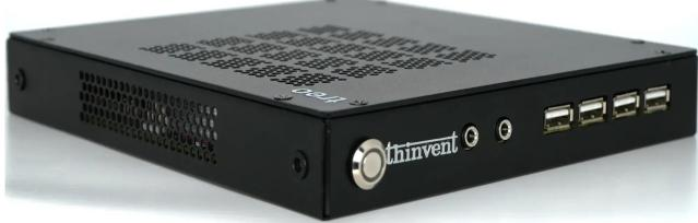
Thinvent® Treo Mini PC, Intel® processor N100 (4 core, up to 3.4 GHz, 6 MB cache), 8GB DDR4 RAM, 32GB SSD, 12V 5A Adapter, No WiFi, Thinux™ Embedded Linux, Thinvent® Keyboard and Mouse set
